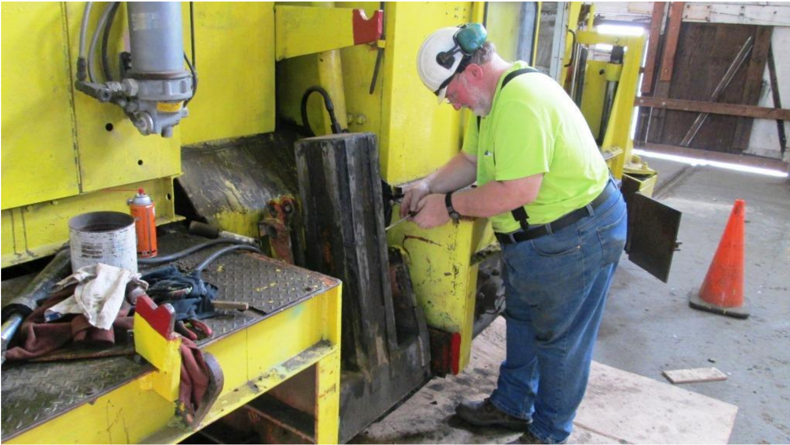
Frank scraping old grease and grime off the pivot arm of the ballast regulator
