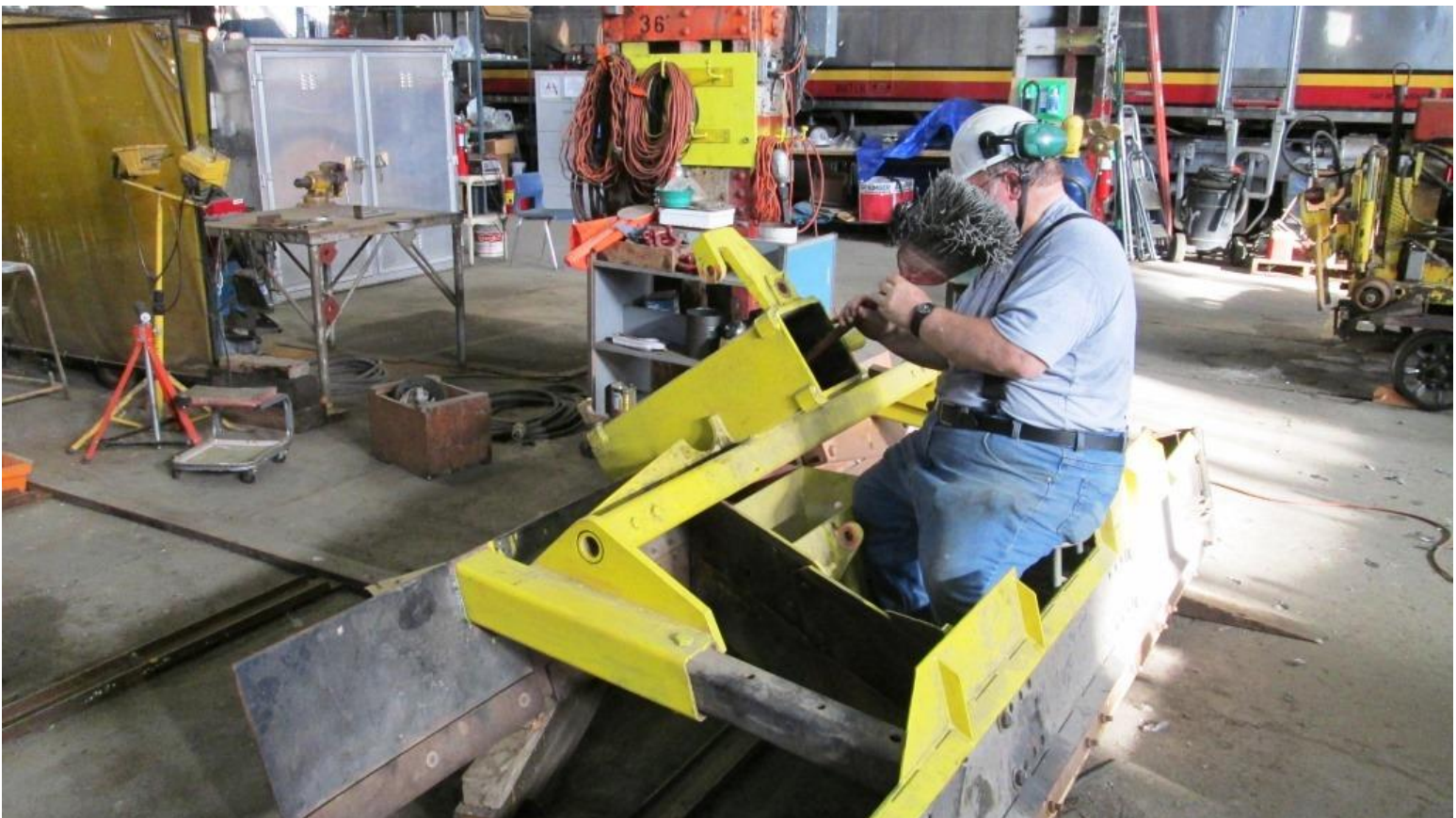
A chimney sweep? Nope, it's Frank cleaning out the slide pocket of the regulator's wing
